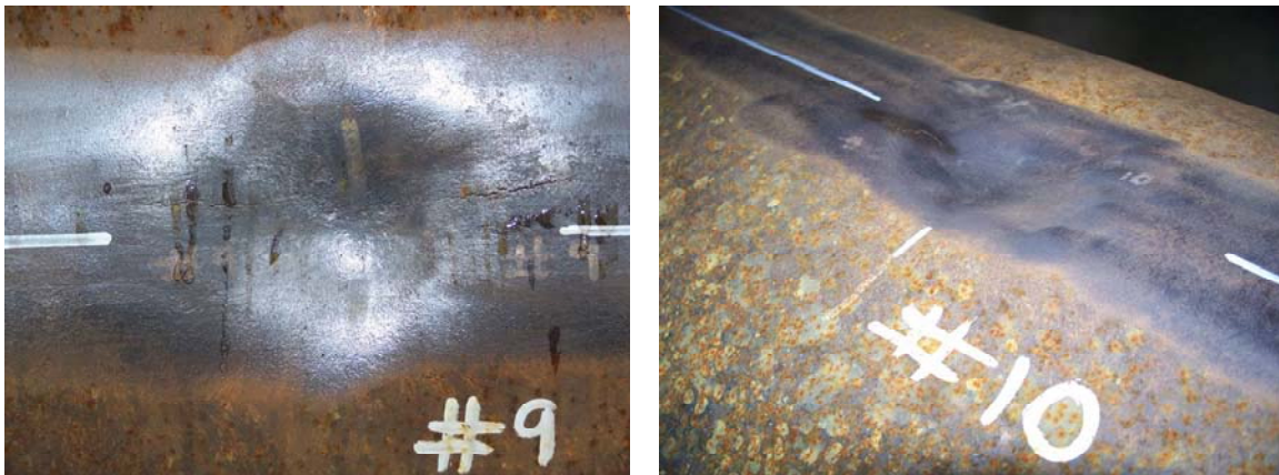
Figure 8 – Photographs of dents from PRCI test samples
