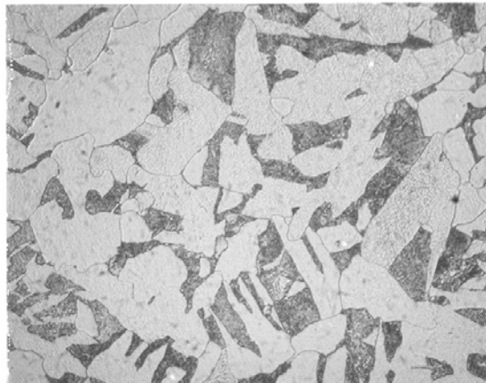
Figure 4 - Carbon steel microstructure observed on a metallurgical replica.
