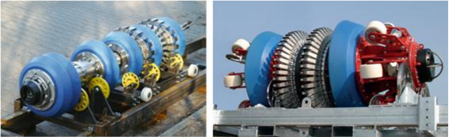
FIGURE 1: ROGEO XT TOOLS WITH TWO MEASUREMENT PLANES (100% CIRCUMFERENTIAL COVERAGE) LEFT: 16-INCH TOOL WITH PULL UNIT AND TWO MEASUREMENT UNITS RIGHT: 42-INCH SINGLE BODY TOOL WITH WHEEL SETUP
