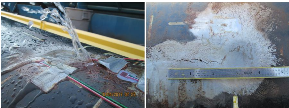
FIGURE 6: DENT FAILURE AFTER 39,800 CYCLES
