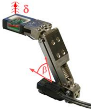
FIGURE 2: COMBINATION OF CONVENTIONAL MECHANICAL CALIPER CONCEPT ( \beta ) WITH A TOUCHLESS OPERATING PROXIMITY SENSOR ( \delta )
