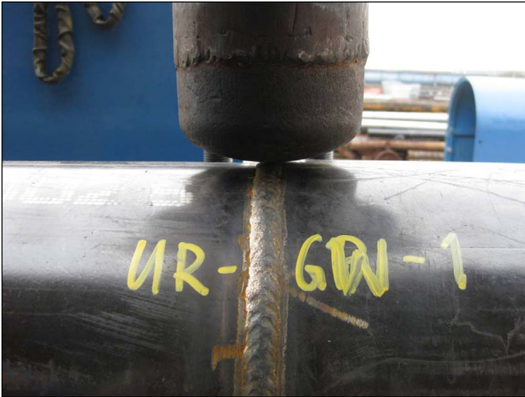
Figure 3 – Close-up view on indenter on girth weld
