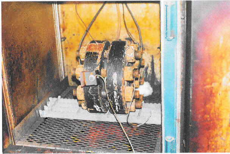
Figure 7 Flange assembly located in heating and cooling chamber
