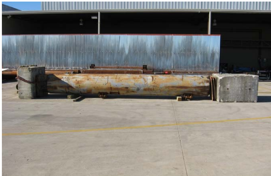
Figure 3 – Burst Test Set-Up
