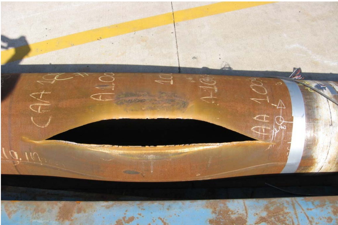
Figure 10 – Failure in Sample #2 (Girth Weld)
