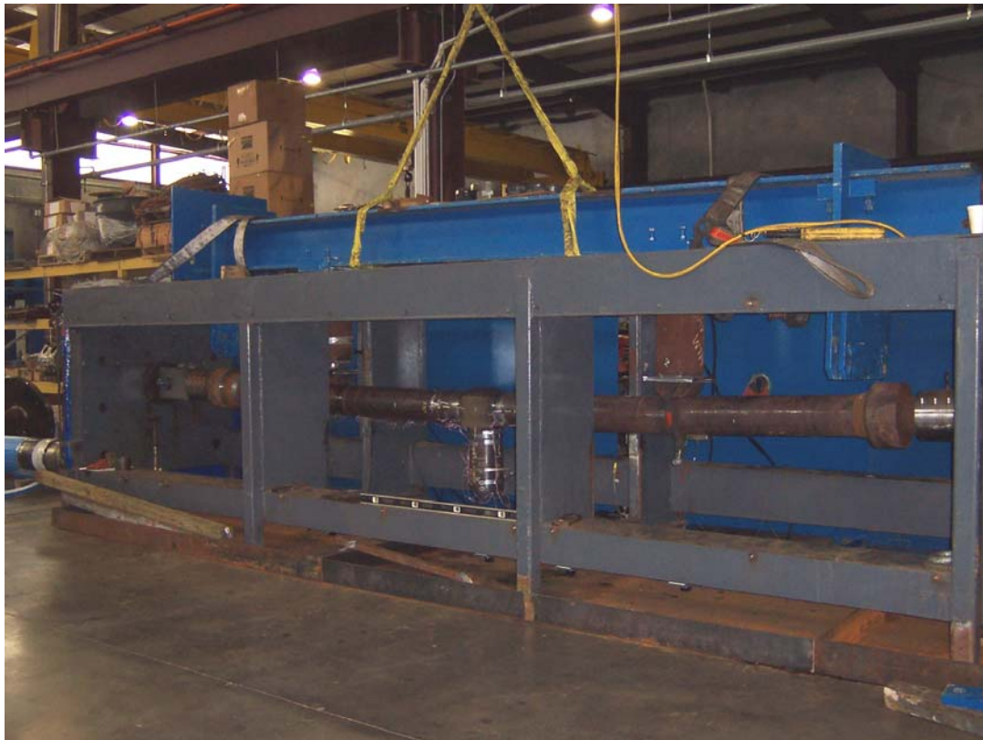
Figure 6 – Load frame used for pressure-tension-bend testing
