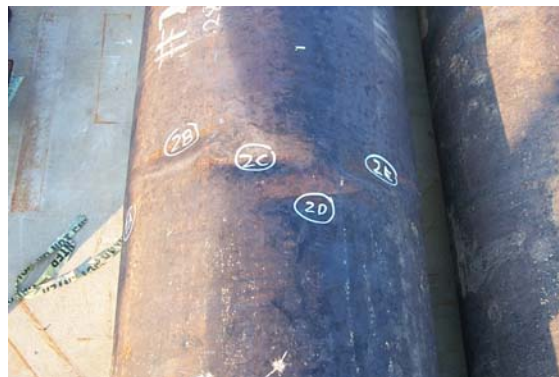
Figure 1 – Photo of 36-inch diameter pipe with 2% wrinkles
