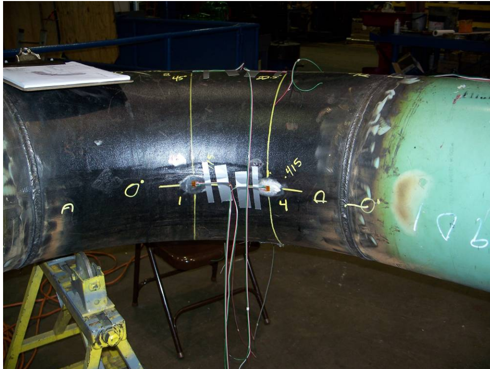
Figure 11 – Photograph of strain gages being installed on the elbow test assembly
