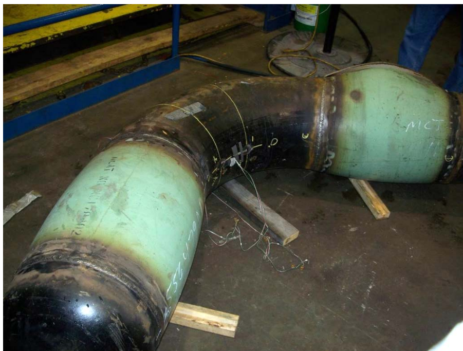
Figure 12 – Photograph of the elbow after burst testing
