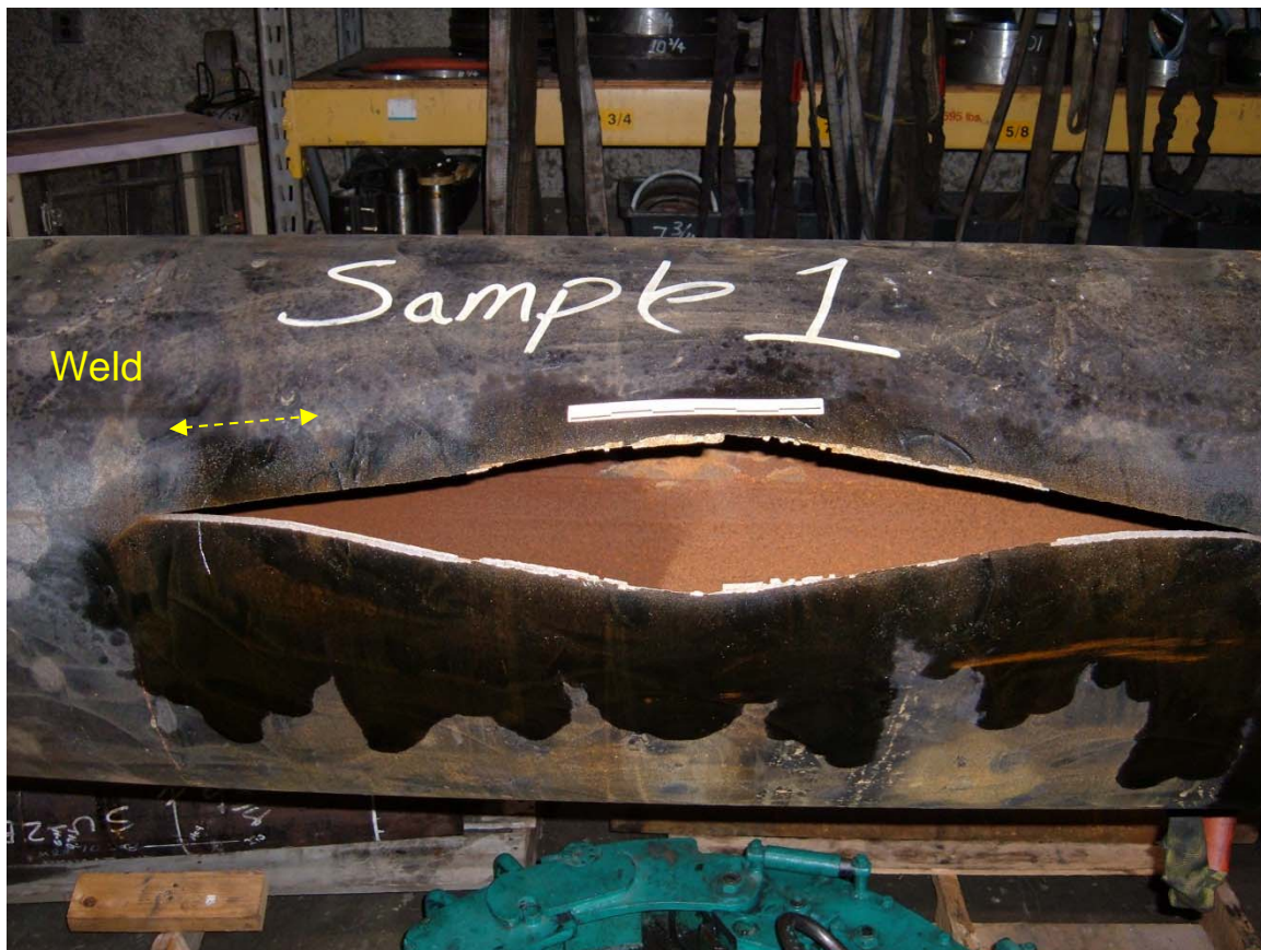
Figure 5 - Hydrostatic test rupture in Sample #1 The location of the longitudinal seam weld is also shown.
