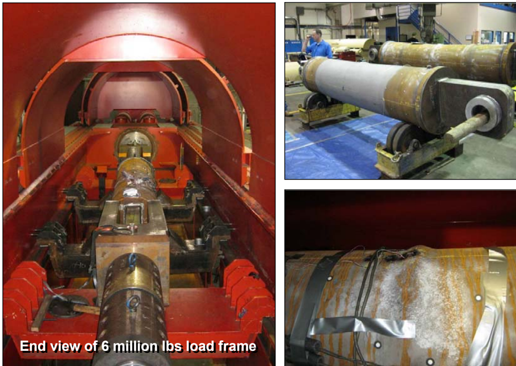
Figure 7 – Photographs showing testing set-up for wrinkle bend testing
