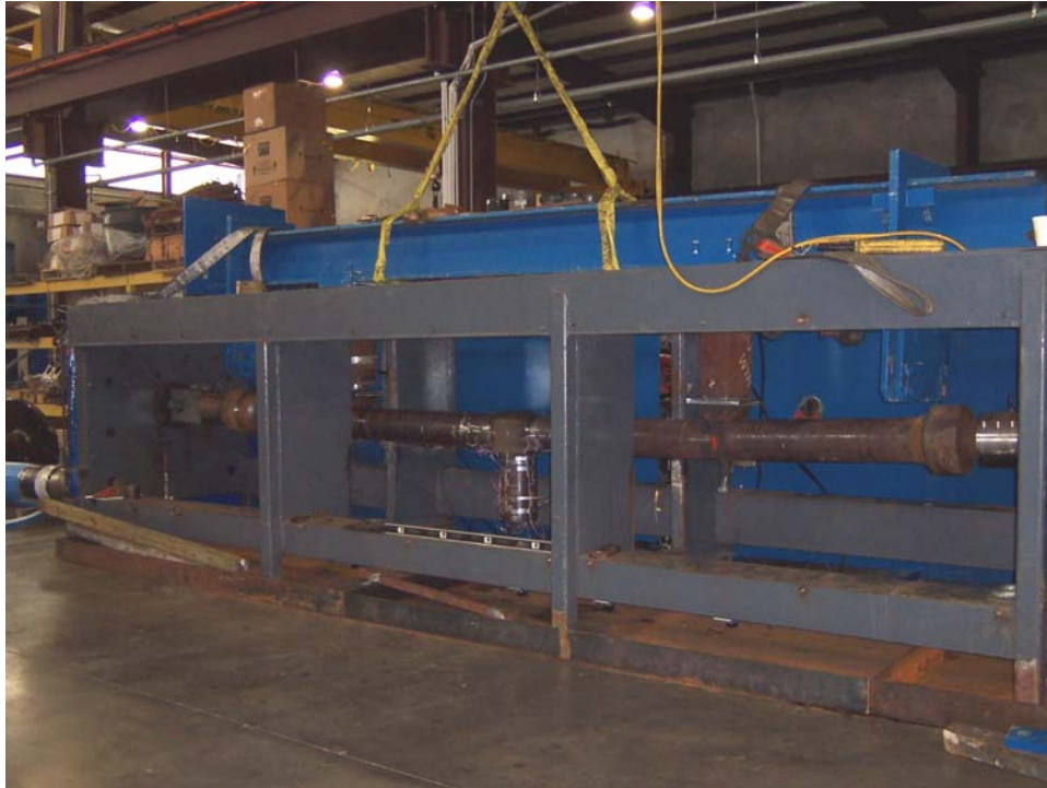
Figure 10 – Load frame used for pressure-tension-bend testing
