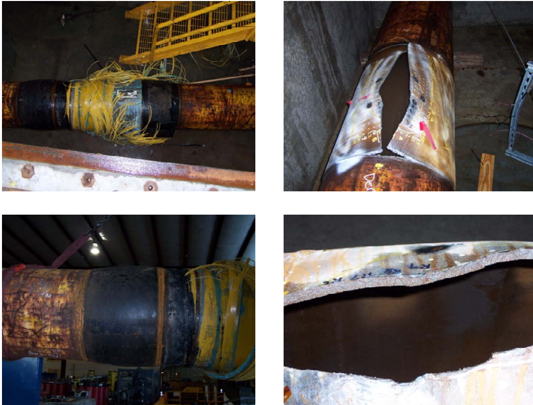
Figure 8 – Photographs from two burst tests that included repaired and unrepaired dents (the two left photos show a dent repaired using the Clock Spring composite repair system)
