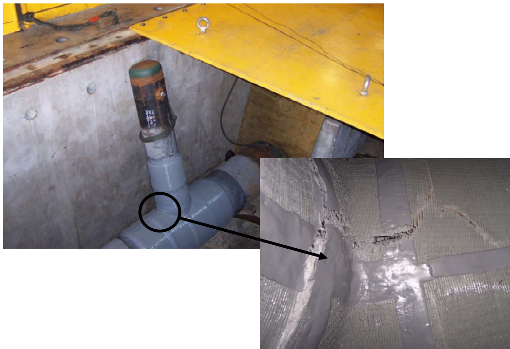
Figure 16 – Leak that developed in composite-reinforced branch connection
