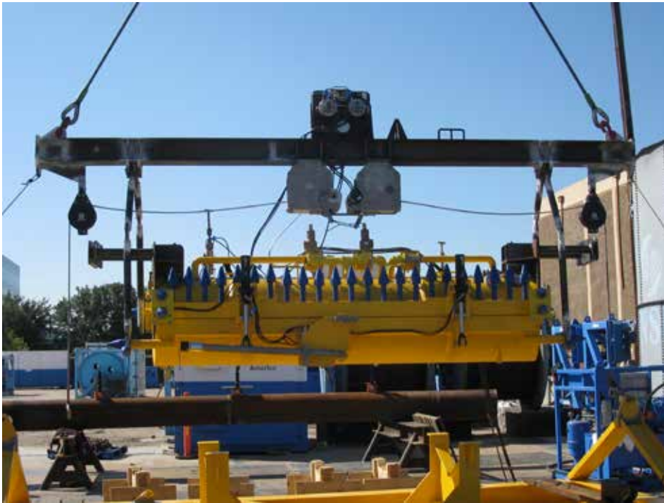
Figure 3 – Grout Sleeve and Spreader Bar during Factory Acceptance Testing
