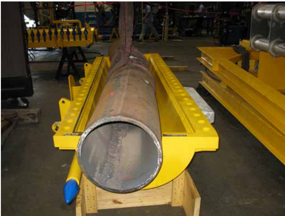
Figure 8 – Fit-up of test pipe fabricated from Metrology Tool measurement
