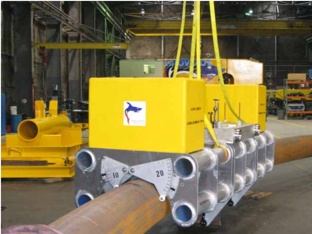
Figure 7 – Metrology Tool landed on test pipe
