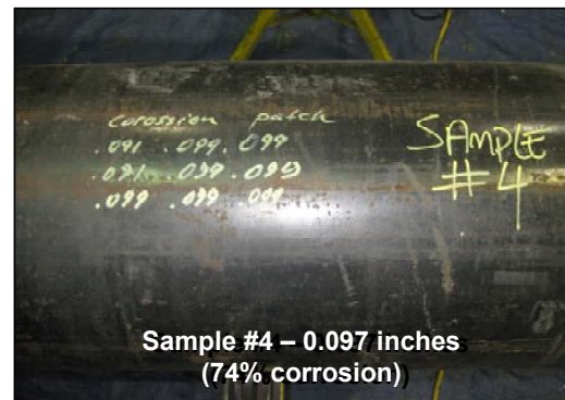
Figure 6– Photographs showing machined corrosion depths
