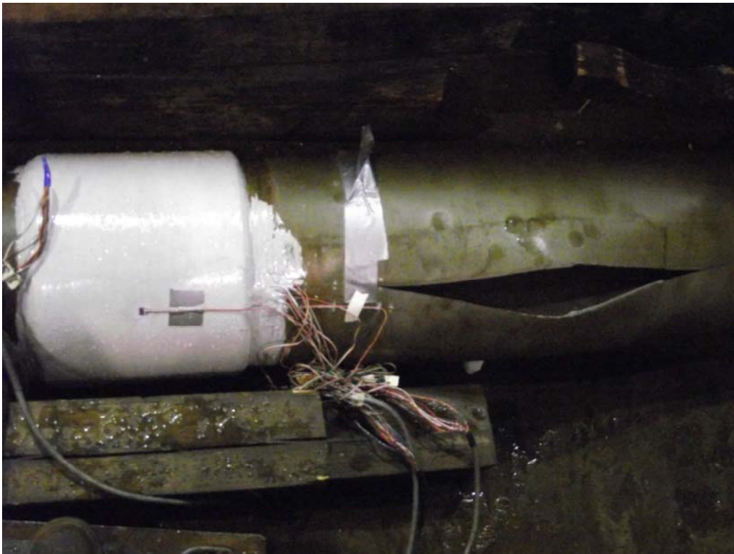
Figure 3 – Photograph of failure in 75% corrosion burst test sample
