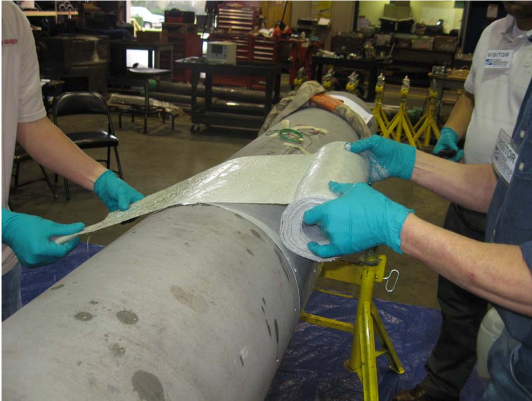
Figure 2 – Installation of composite repair on 75% corrosion burst test sample
