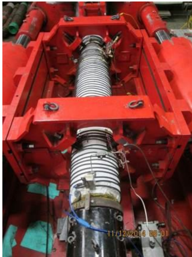
Figure 7: Compression sample in load frame
