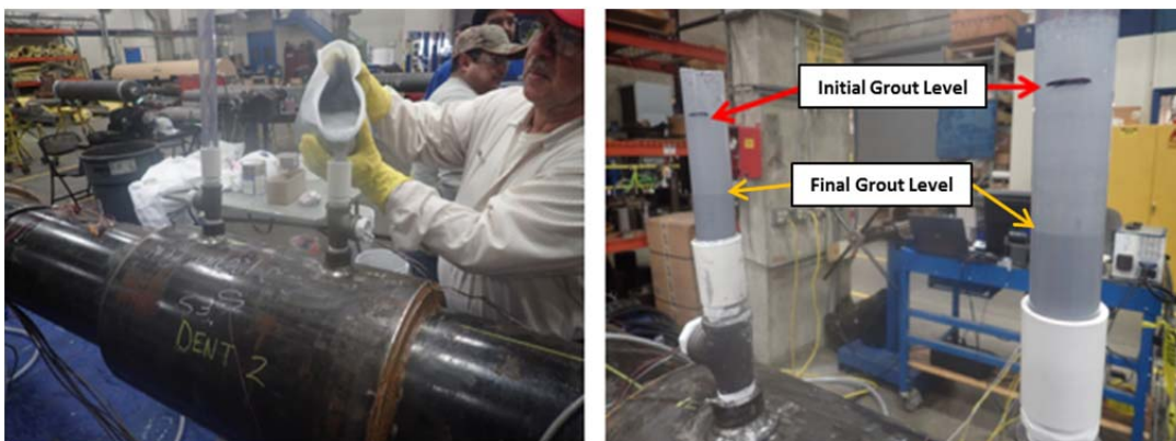
Figure 8: Dent #2, Armor Plate Epoxy Grout Installation
