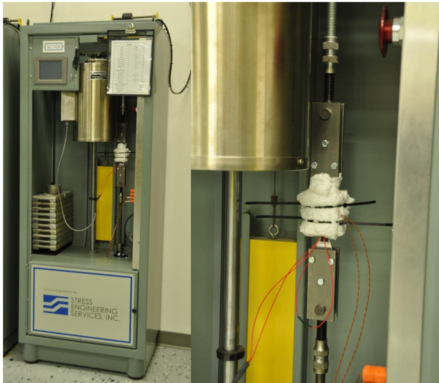
Figure 1: M3 Creep Frame / Loaded creep-rupture sample
