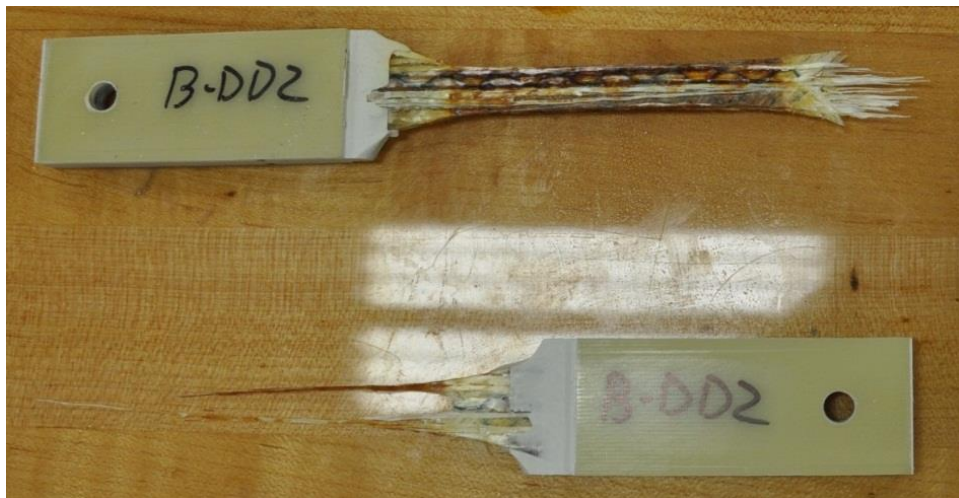
Figure 7: System F creep-rupture – post-failure
