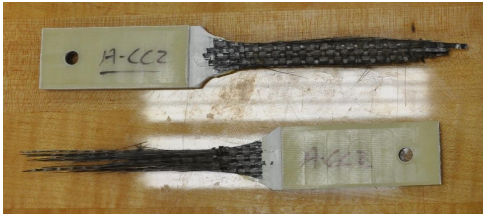
Figure 5: System E creep-rupture specimen – post failure
