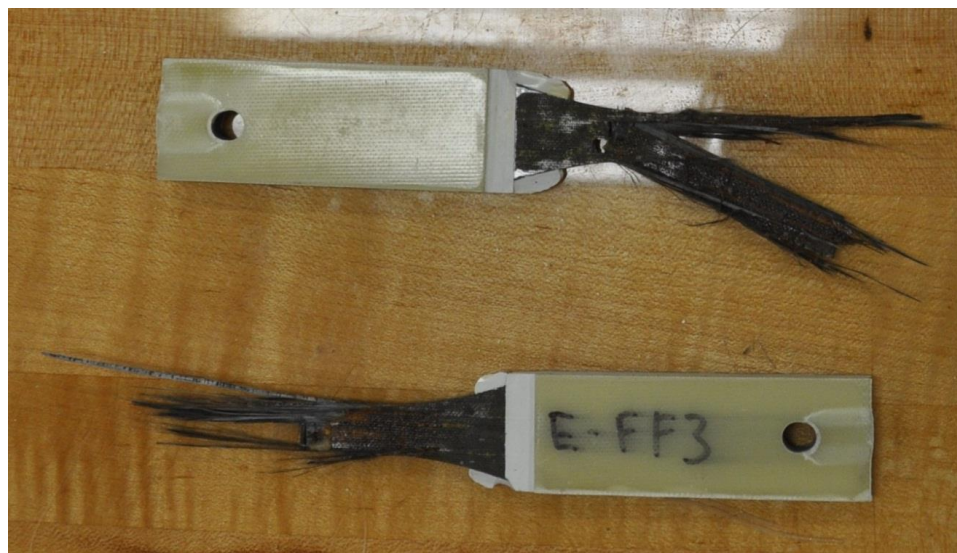
Figure 4: System D creep-rupture specimen – post failure
