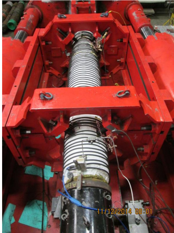
Figure 3: Photograph of full-scale compression test setup
