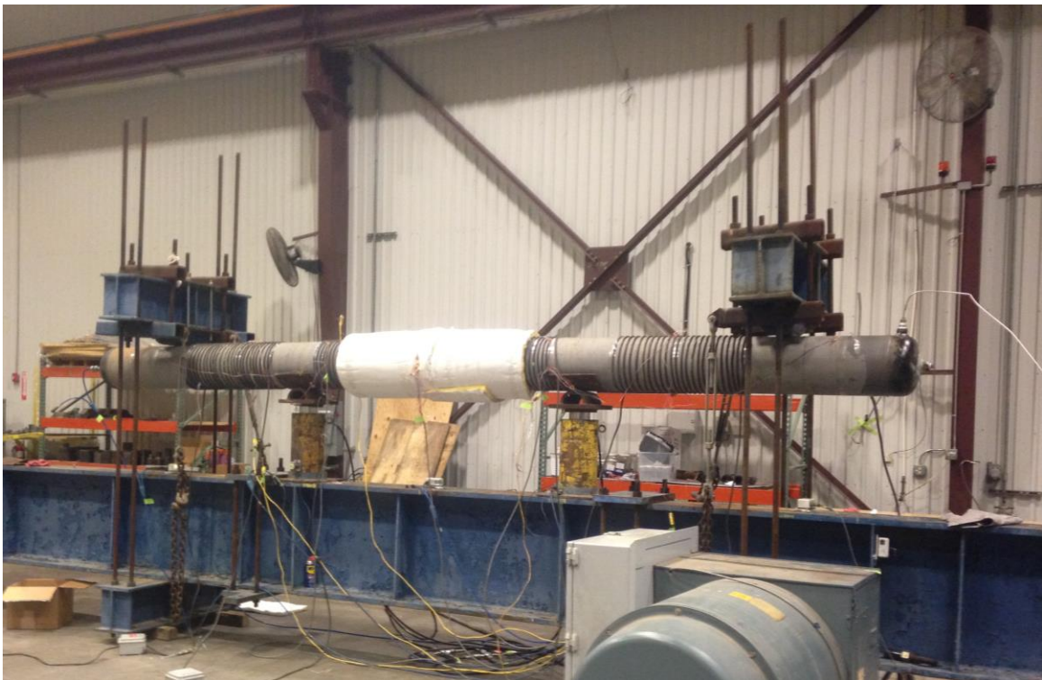
Figure 4: Photograph of full-scale bend test setup
