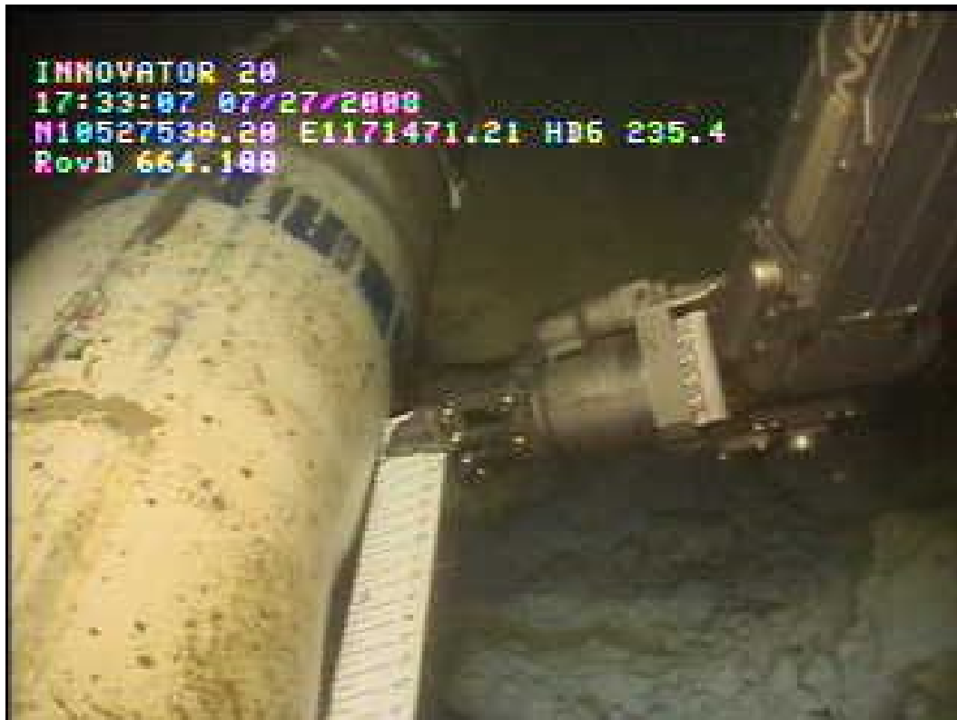
Figure 1 – ROV-assisted measurement of dent using a straightedge
