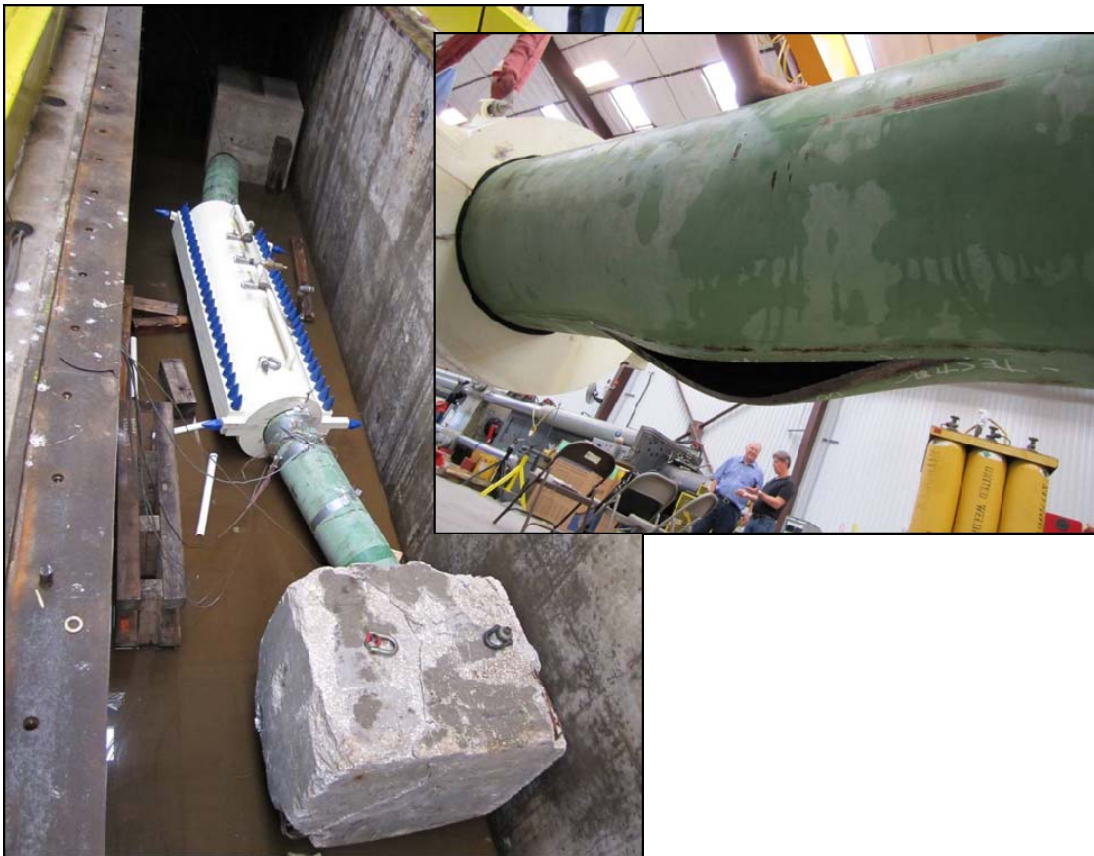
Figure 11 - Photograph showing burst test for repaired sample with failure outside of sleeve
