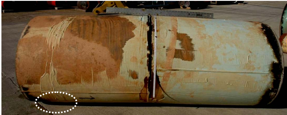
Figure 2 – Photograph and two sketches showing ruptured pipe section as received (Arrow (circled) indicates direction of flow)
