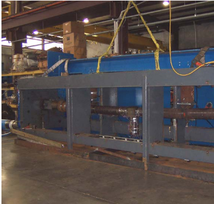
Figure 9 – Load frame used for pressure-tension-bend testing
