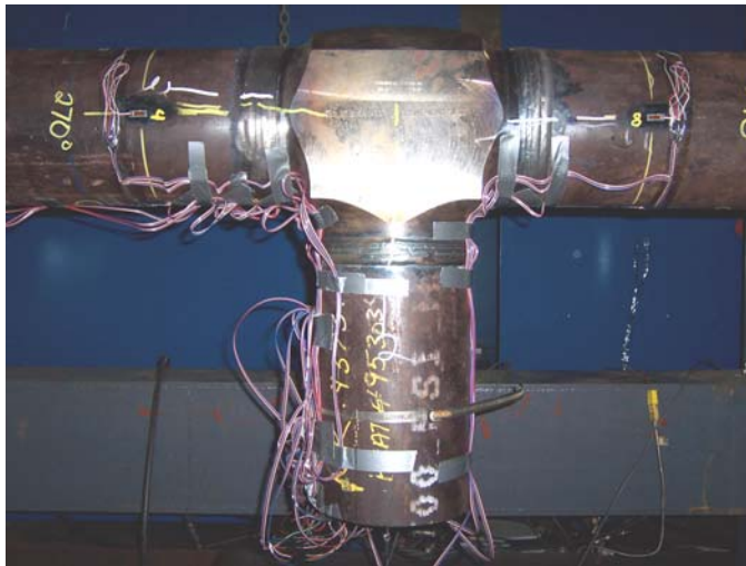
Figure 6 – Close-up photo of tee showing installed strain gages
