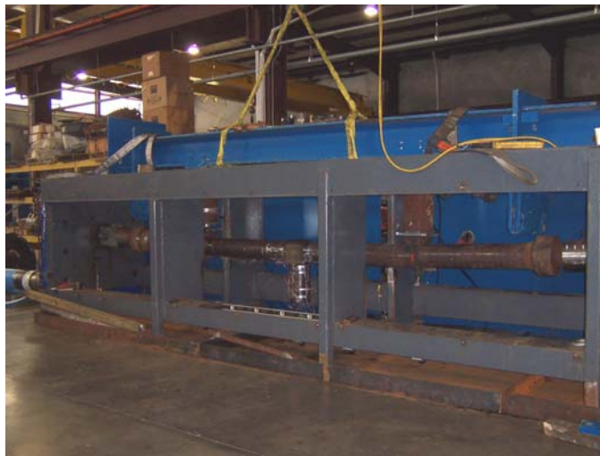
Figure 9 – Photo showing overall view of test assembly (blue I-beam on top used to provide reaction support to bending cylinders)
