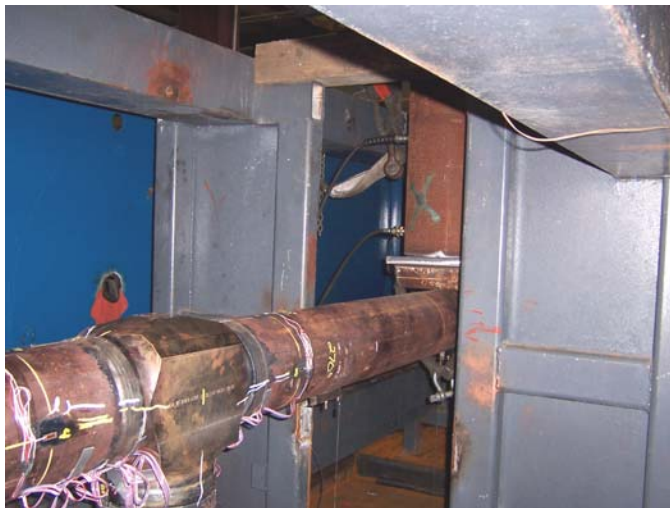
Figure 8 – Photo from center of sample showing bending fixture
