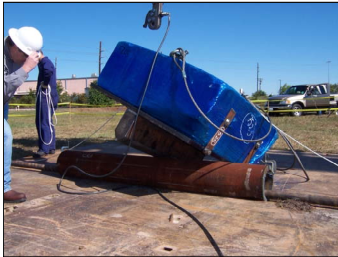
Figure 13 - Photographs from 1 MJ full-scale drop test
