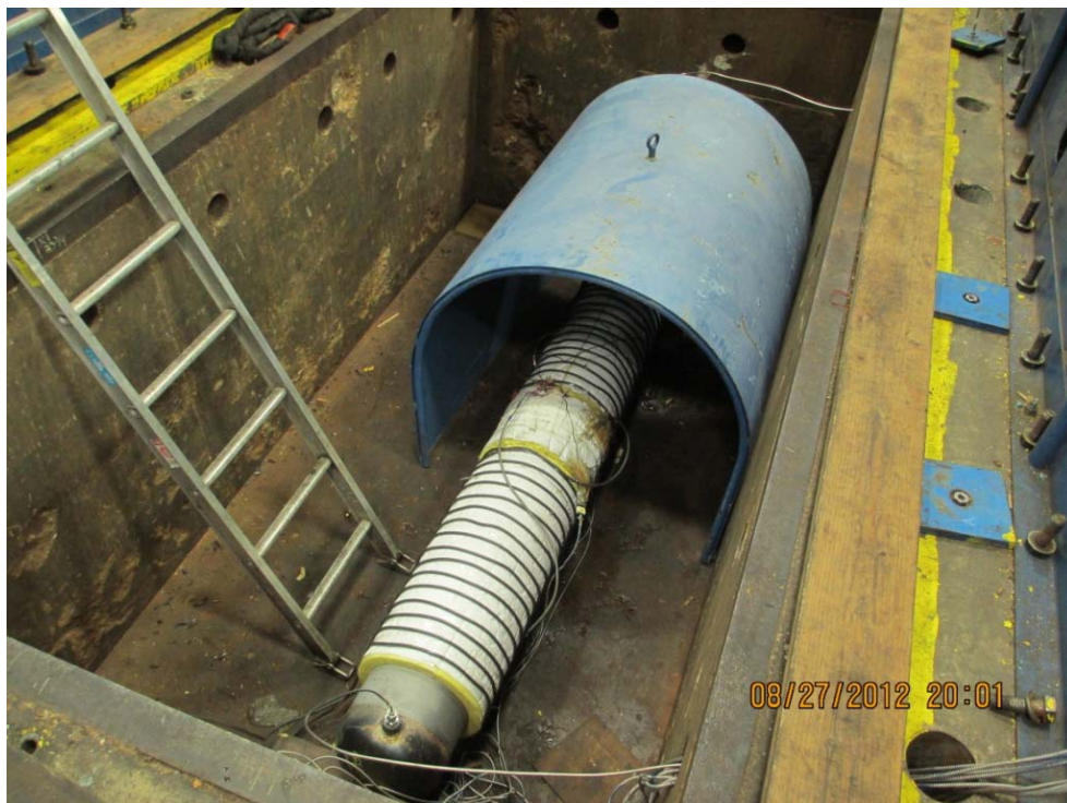
Figure 11 – Photograph of sample in test pit with insulation and induction heating coils
