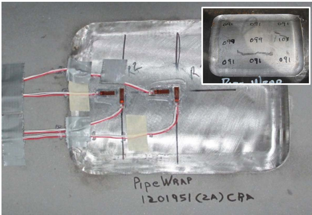
Figure 9 – Close-up view of the machined region of the pipe sample
