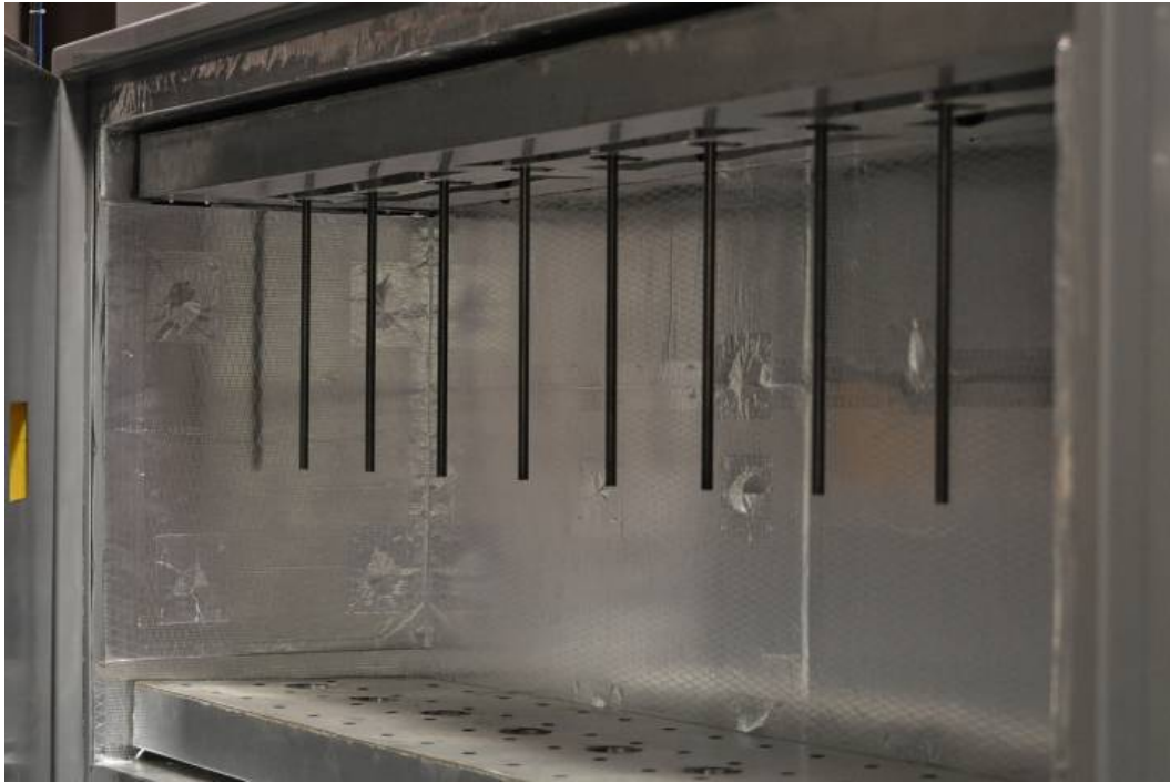
Figure 6 – Close-up view of the creep test facility showing loading chamber
