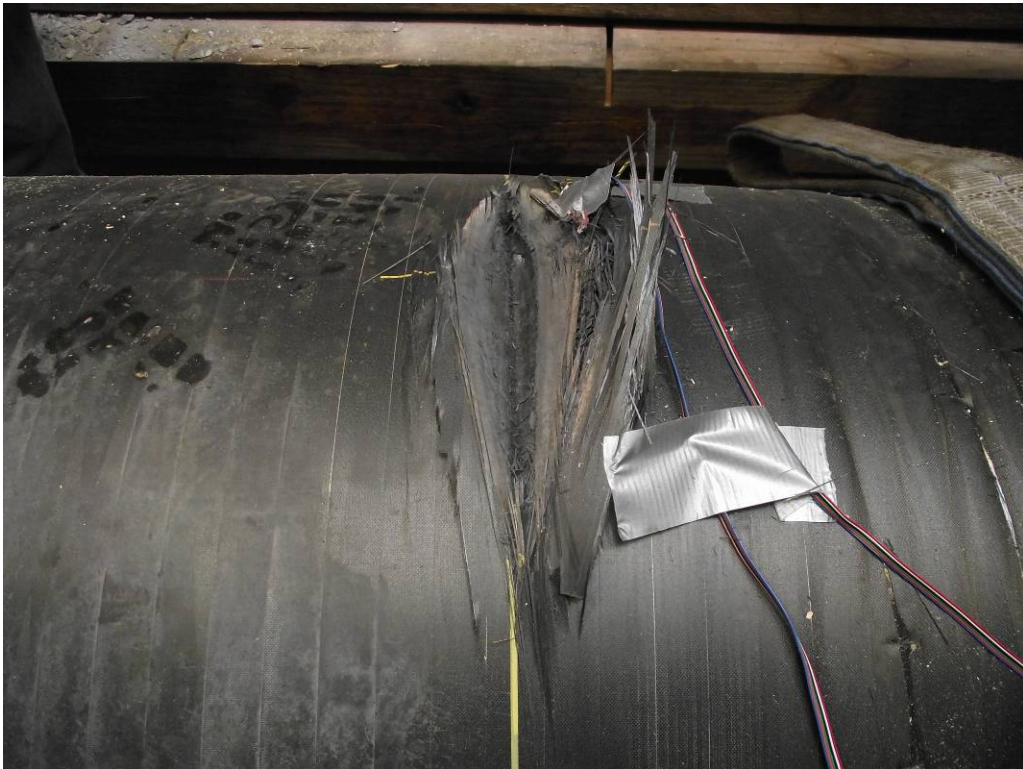
Figure 8 – Photograph of Impact Damage at First Trap
