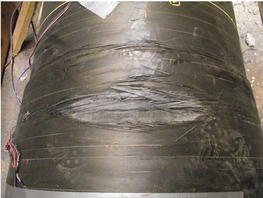
Figure 10 – Photograph of Impact Damage at End Connector Weld
