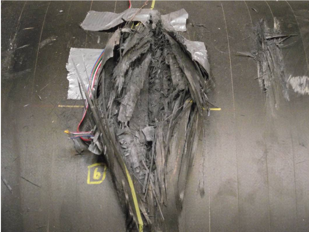
Figure 9 – Photograph of Impact Damage at Center Weld Location
