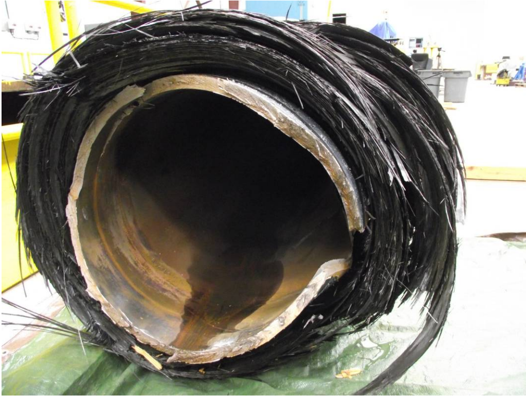
Figure 13 – End View of Burst Failure of SN3
