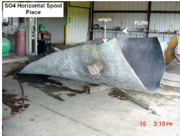
Figure 1 - Horizontal spool piece showing fatigue-cracked seam weld
