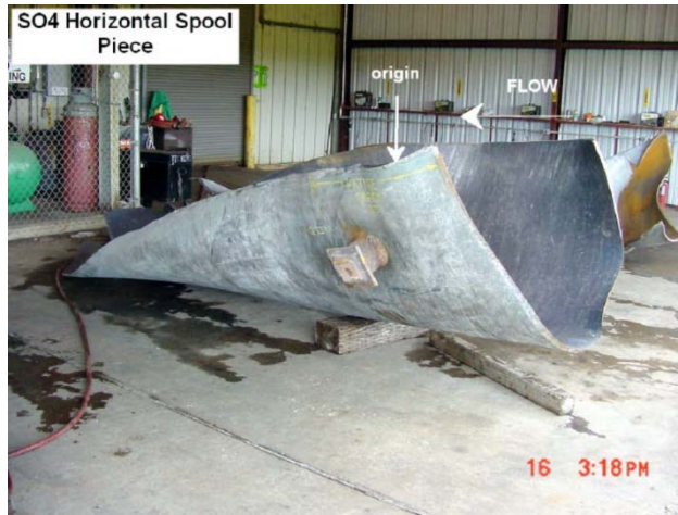
Figure 2: Horizontal spool piece showing fatigue-cracked seam weld
