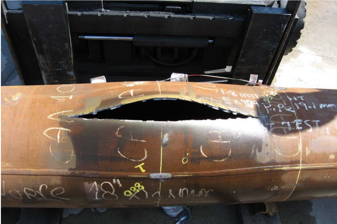
Figure 9 – Failure in Sample #1 (Base Pipe) indicating ductile failure mode
