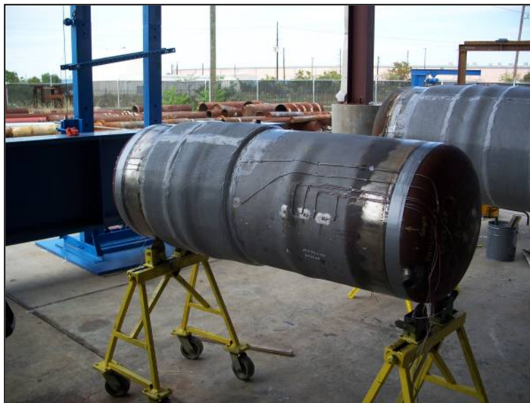
Figure 3 – Photo showing completed installation of composite material
