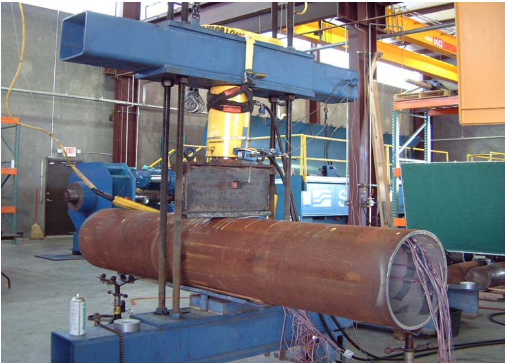
Figure 6 – Photograph of dent installation rig [15]
