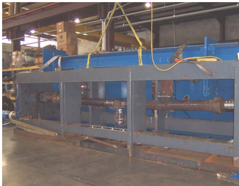
Figure 2 – Images of pressure-tension-bending load frame test set-up
