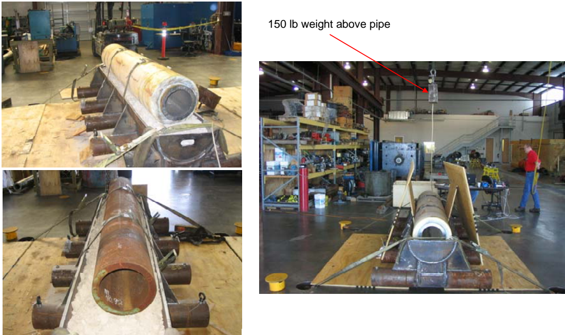
Figure 3 – Experimental set-up for sub-scale testing
