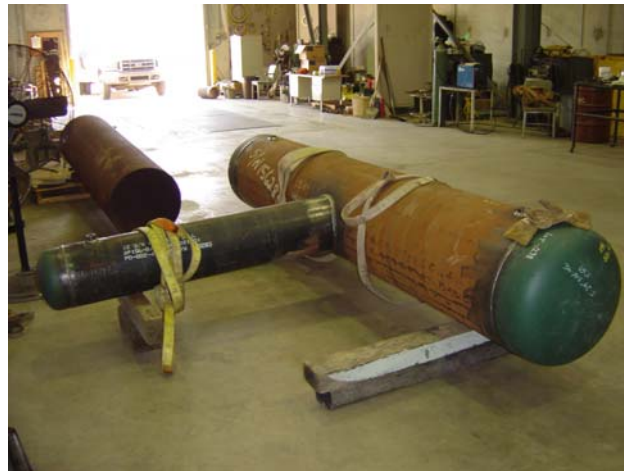
Figure 1 - Photograph of branch connection prior to reinforcement
