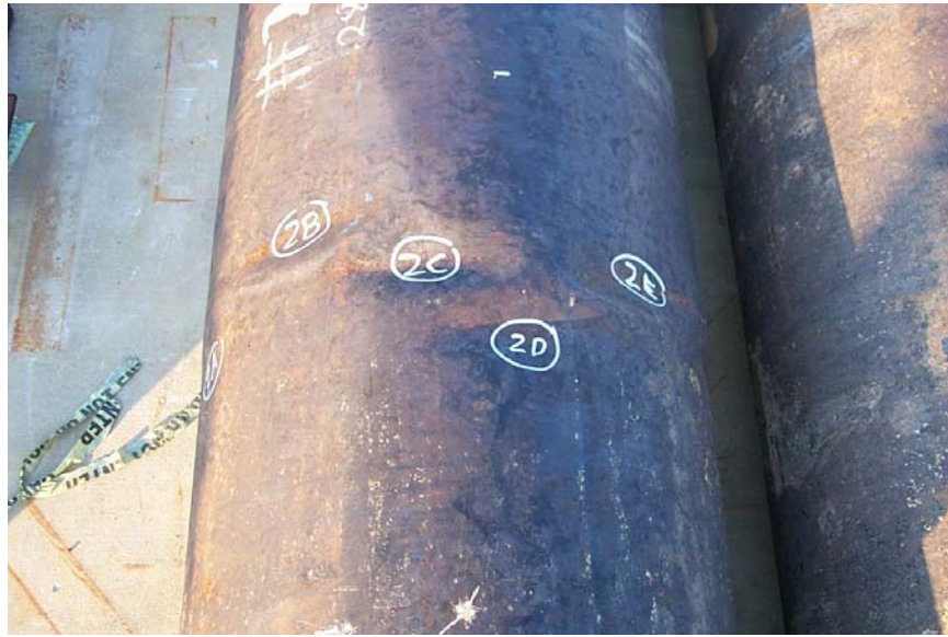
Figure 1 – Photo of 36-inch diameter pipe with 2% wrinkles
