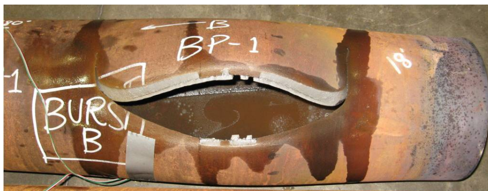
Figure 6A – Photographs of Burst Test Samples (Sample BP-1B)
