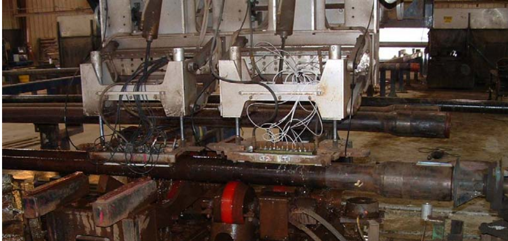
Figure 2 – Full-Length Ultrasonic Test (FLUT) Inspection Set-up
