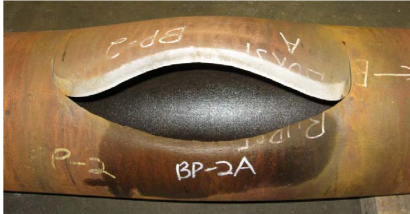
Figure 6B – Photographs of Burst Test Samples (Sample BP-2A)
