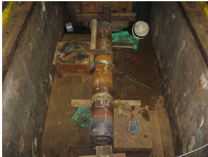
Figure 5 – Burst Test Sample in SES Test Pit
