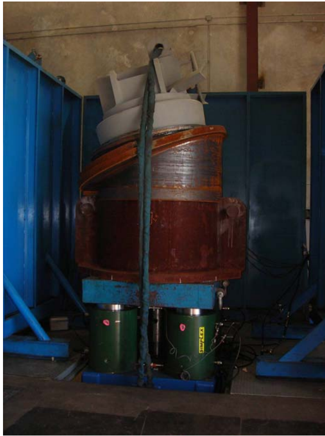
Figure 7 - Test Set-Up for 10-inch/8-inch Cross-Haul Bucket
