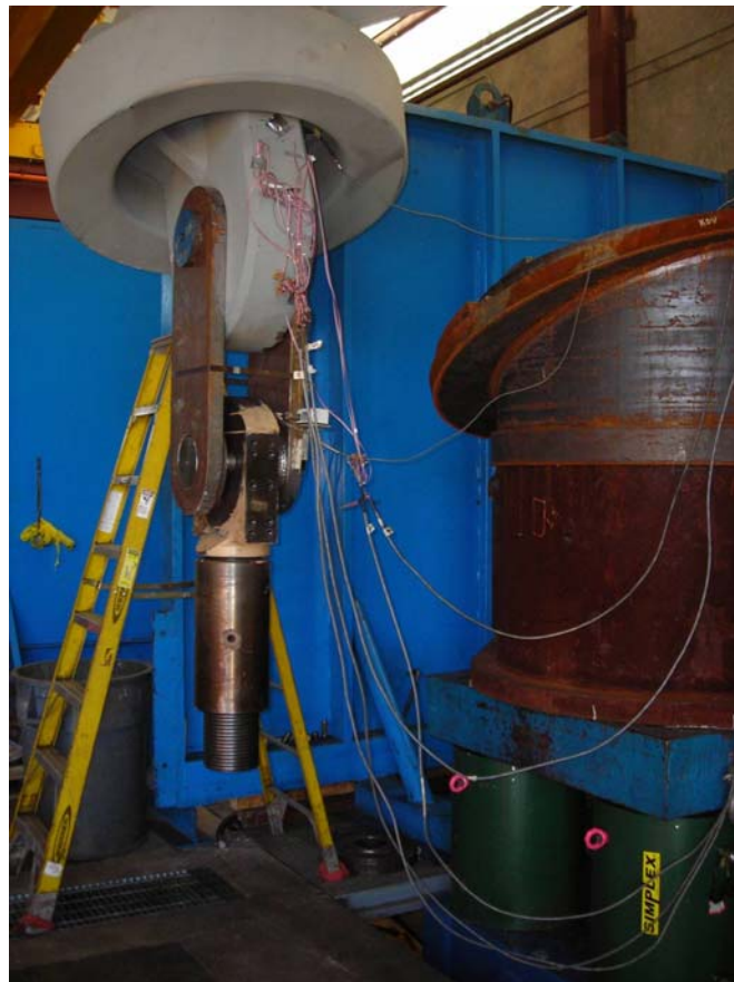
Figure 6 - Assembled Cross-Haul Bucket and Reaction Shaft
