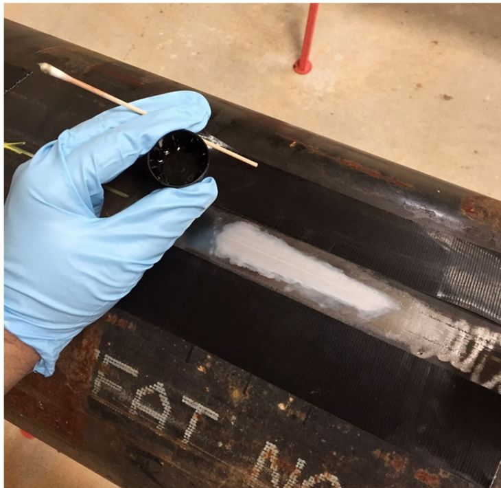
Figure 2: Macro-etching to locate the ERW bondline
