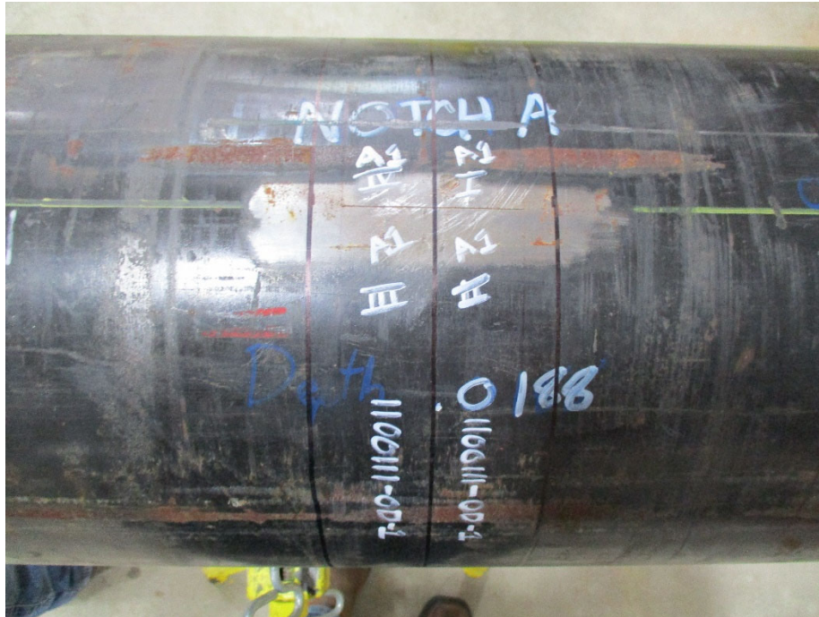
Figure 3: Example of how notches were labeled and sectioned
