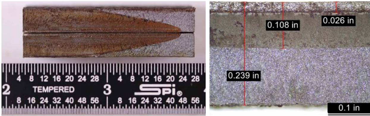
Figure 7: Cracks on Sample 2: (a) Notch C2; (b) Notch C1
