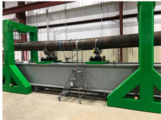
Figure 14: Photographs showing set-up of a wrinkle bend test in the bending load frame
