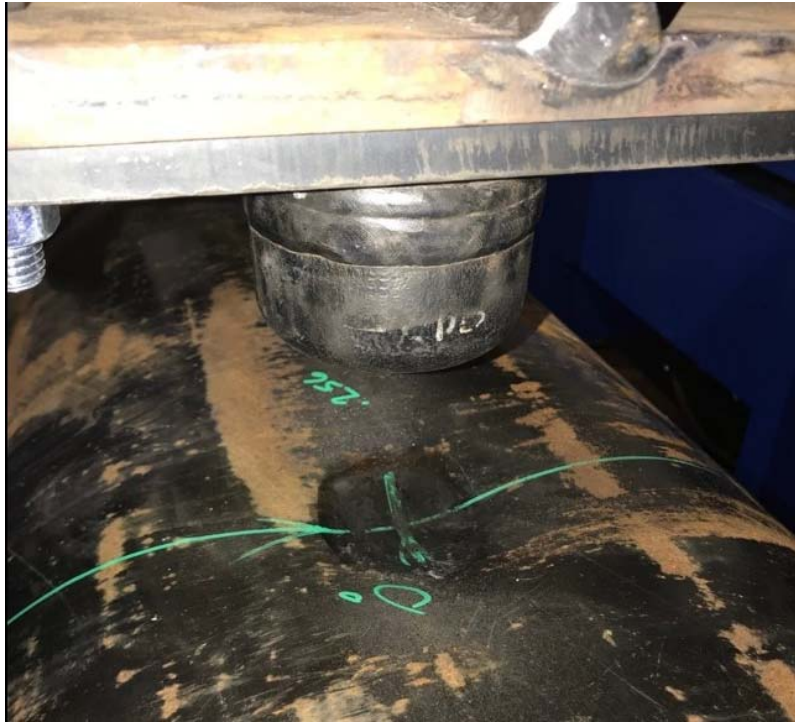
Figure 15: View of simulated dent after indenter removal
