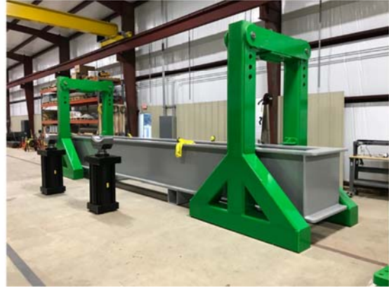
Figure 13: Photographs showing set-up of the 3.5 million ft-lb bending frame
