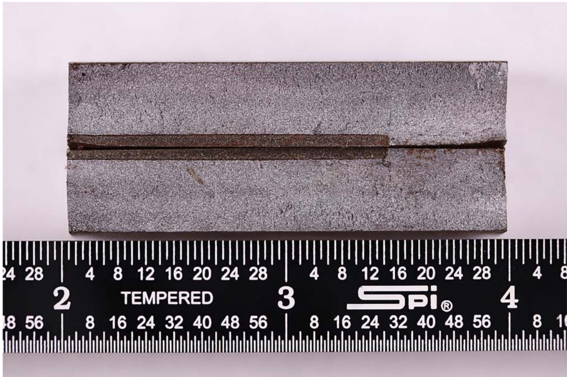
Figure 9: Meridional post-test sectional view of the EDM Notch C
