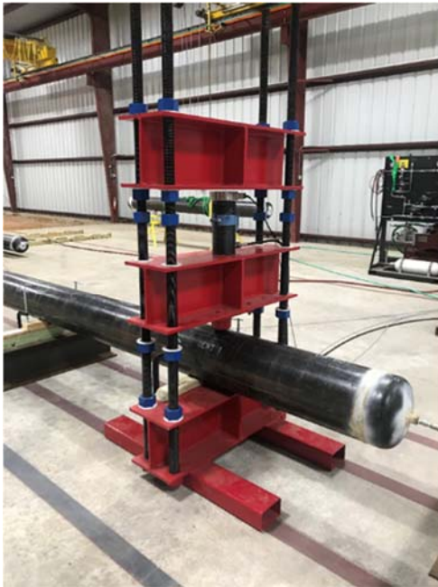
Figure 5: Photographs showing the dent installation test rig
