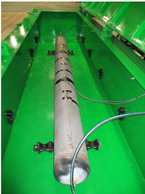
Figure 6: Photographs the dent test sample and associated fatigue crack
