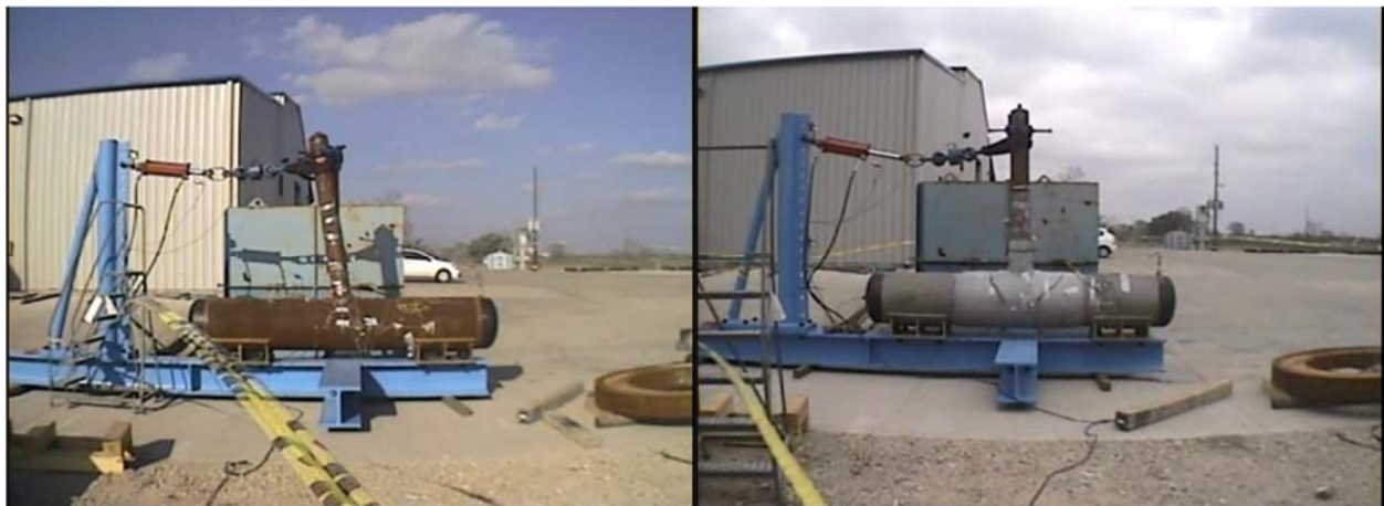
Final displacements for in-plane unreinforced (left) and reinforced (right) bending tests
