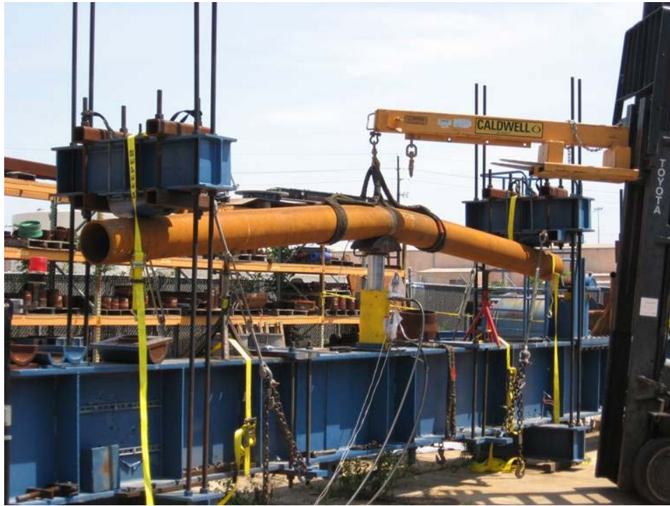
Figure 7: Photograph showing bending test set-up to validate fiber optic technology (Case Study #3)
