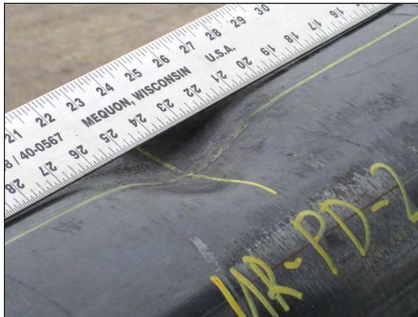
Figure 8: Photograph showing plain dent test sample after indentation
