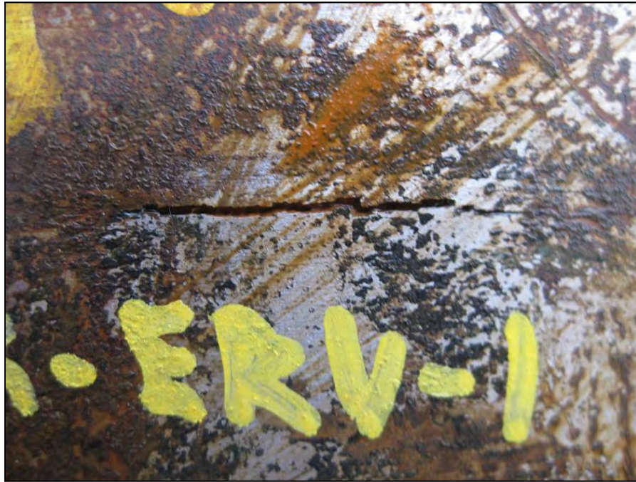
Figure 9: Photograph showing typical fatigue crack in dented test samples
